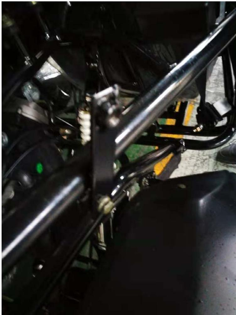
15.2、 Clamp  $\phi 32$  stainless steel embrace hoop on the roll cage rear, screw the lower front part of the rear plastic plate on the front position of rear cargo rack with M6\*16 bolts, connect the hoop and the front upper part of the rear plastic plate with M6\*20 bolts and M6 flange nuts.
