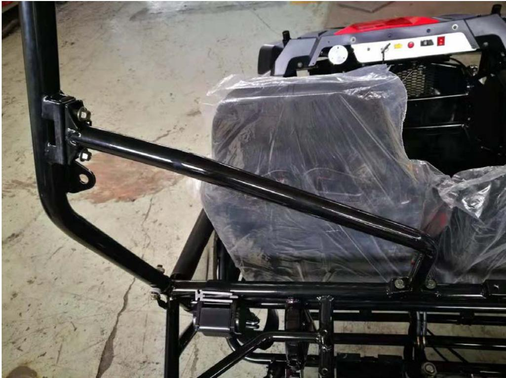
11、 Assemble roll cage front: put front side of roll cage bar onto the connection rods on frame, fixing with bolt M8x55, R-washer and M8 nut. Then put back side onto the connection rods of roll cage rear, fixing with bolt M8x55, R-washer and M8 nut. The bolt is screwed on but not tightened.
