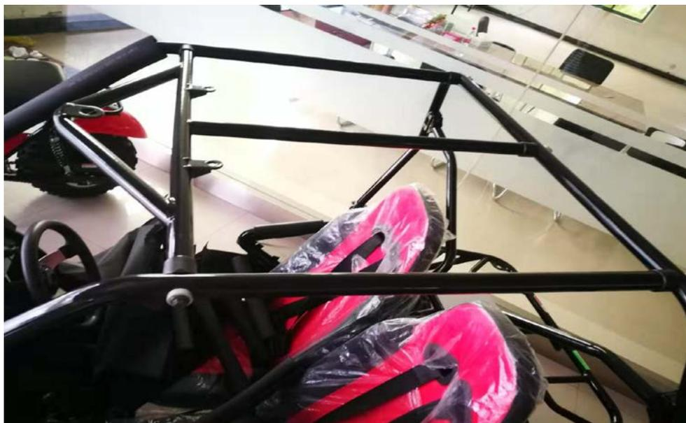
13、 Tighten the mounting bolts in the assembly sequence of 9, 10, 11 and 12, and the torque is 22-29NM.
