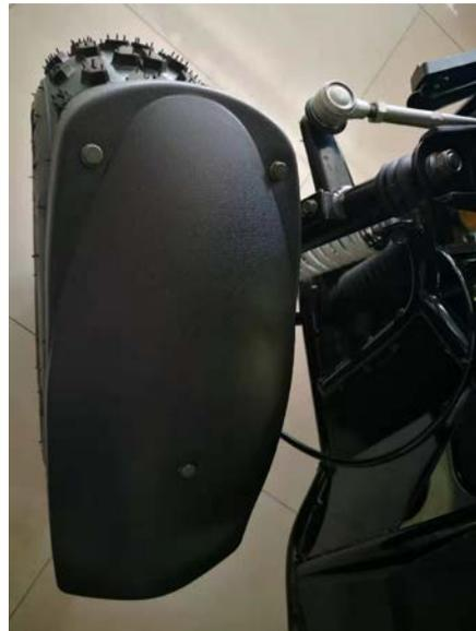
8、 Assemble the front wheel: fit the front wheel onto the hub, screw the locking nut M10x1.25 tightly with 37-44NM. Use a crisscross sequence until they have reached their proper torque value. Then cover the hub cover.
