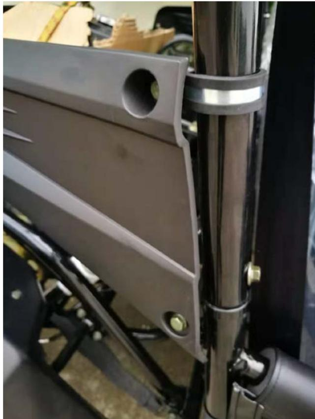
15.3、 Use M6\*20 bolts and M6 flange nuts to connect and install the upper part of the rear plastic plate and the back part of the rear plastic plate. Tighten all bolts with a tightening torque of 11-16NM.
