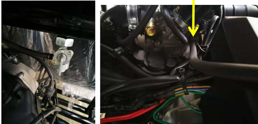
18.2、 Connect the oil tank dumping check valve tubing to the air filter.
