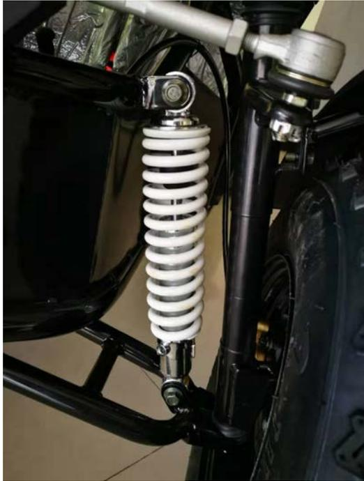
7、 Assemble the front fender: take down the bolts M6\*16 on the strut, assemble the fender, fix the bolt with torque 11-16NM.
